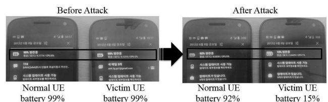
Fig. 10: Result of battery depletion attack
