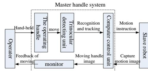
Fig. 2: the block diagram of the master handle subsystem
