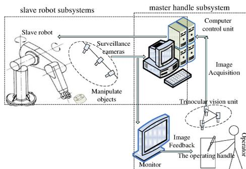
Fig. 1: The structure of Master-slave robot system
