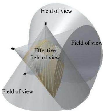
Fig. 4: the overlapping field of three camera views
