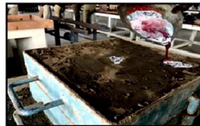
Fig. 3: Pouring of Al (6063) molten metal in Sand Casting setup.
