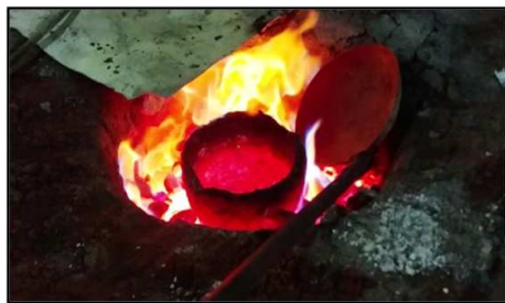
Fig. 2: Al (6063) melts in crucible furnace.
