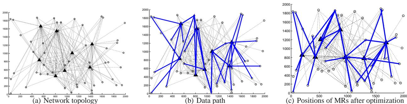
Fig. 1: A wireless network with regular nodes and MR nodes
