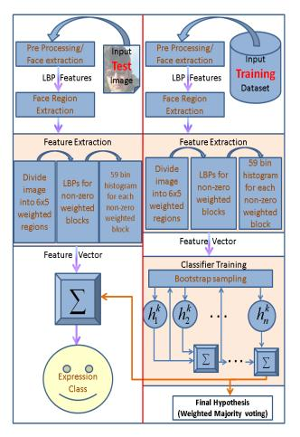
**Fig. 2:** Block diagram of the proposed system: right side represents the training process and left side represent the testing process
