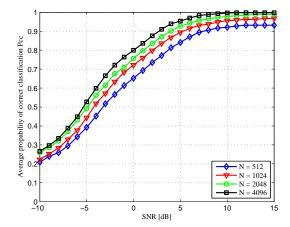
**Fig. 2:** Average probability of correct classification versus SNR for different observation interval lengths.
