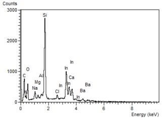
Figure 6: EDAX analysis of Ba-TCNQ sample.
