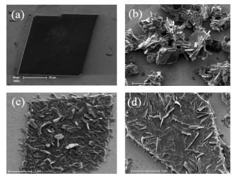
**Figure 7:** (a) SEM image of a single crystal of TCNQ present on a TCNQ-modified ITO electrode prepared via the drop casting method. (b) SEM image of Ba[TCNQ]<sub>2</sub> formed by reductive electrolysis for 10 min at -0.10 V of TCNQ-modified ITO.
