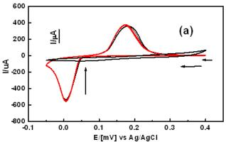
**Figure 1:** Cyclic voltammograms obtained with a scan rate of 20 mV s<sup>-1</sup> for the fifth cycle of the potential over the range of 0.45 to -0.1 V at (a) bare GC surface and (b) TCNQ-modified GC disk electrode (mechanical attachment) in contact with 0.1 M Ba(NO<sub>3</sub>)<sub>2(aq)</sub> electrolyte.
