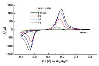
**Figure: 3:** Cyclic Voltammograms obtained with TCNQmodified GC electrode (mechanical attachment) in contact with 0.1 M Ba(NO<sub>3</sub>)<sub>2(aq)</sub> solution at designated scan rates.
