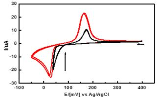
**Figure 4:** Cyclic Voltammograms obtained with TCNQmodified GC electrode in contact with 0.1 M  $Ba^{2+}_{(aq)}$  solution at scan rate of 0.020 V s<sup>-1</sup>.
