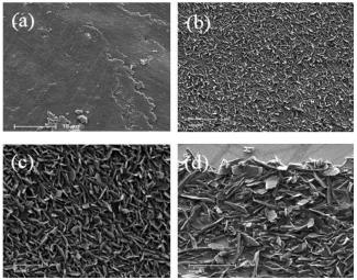
**Figure 8:** (a) SEM image of a TCNQ-modified ITO surface via mechanical attachment method before introduced into the electrochemical cell. (b) SEM image of Ba[TCNQ]<sub>2</sub> micro-sheets formed by reductive electrolysis for 10 min at -0.10 V of solid TCNQ adhered to an ITO electrode surface as image (a) when placed in contact with 0.1 M  $Ba(NO_3)_{2(aq)}$  electrolyte. Images (c and d) are as in image (b) but higher magnifications.
