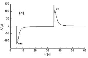
**Figure 5:** Double-potential step chronoamperograms obtained when a GC electrode modified with microcrystals of TCNQ (mechanical attachment) is placed in contact with 0.1 M Ca(NO<sub>3</sub>)<sub>2(aq)</sub>: (a) *i-t* transient obtained when the potential is initially stepped from  $E_i = 400$  to  $E_{red} = -10$  mV for 30 s to induce reduction and then back to  $E_{ox} = 165$  mV to induce oxidation
