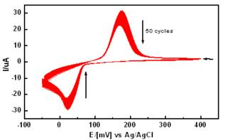
**Figure 2:** Cyclic voltammograms (first 50 cycles of potential) obtained at a scan rate of 50 mV s<sup>-1</sup> when a TCNQ-modified GC electrode prepared via the mechanical attachment method is placed in contact with 0.10 M  $Ba(NO_3)_{2(aq)}$  electrolyte and scanned over the potential range of 0.45 to -0.050 V.
