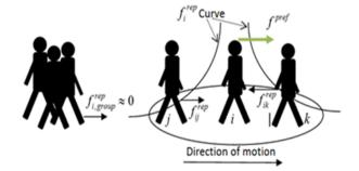
Figure 1 The perception of a pedestrian is represented as a circle centered at the location of the pedestrian himself. The radius of this area and the effects of the inside elements vary according to both the magnitude of  $B^{rep}$  and the weight function W, modeled in Eq. 7.
