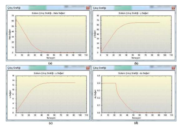
Fig. 10: Screenshots from the graphics viewed after a control process (94 iterations), a) error value, b) Output of system y value, c) The total system/model output u value, d) The change of system/model output du value.
