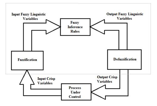
Fig. 1: A typical Fuzzy Logic Control – Fuzzy Control system schema [24].
