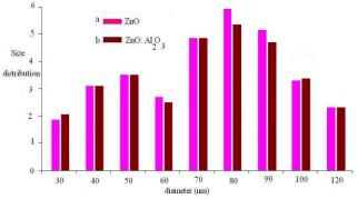
**Fig.3** Particle size histogram of the (a) ZnO and (b) ZnO-Al<sub>2</sub>O<sub>3</sub> nanoparticles.
