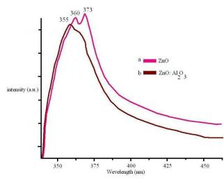
**Fig.5** Solid state absorption spectrum of (a) ZnO and (b ZnO-Al<sub>2</sub>O<sub>3</sub> nanoparticles (λex=320).
