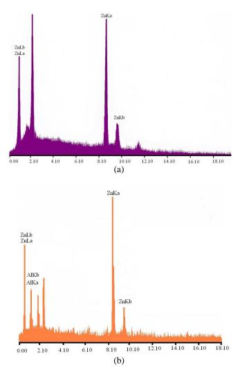
Fig.4 EDAX analysis of the (a) ZnO and (b)  $ZnO-Al_2O_3$  nanoparticles.
