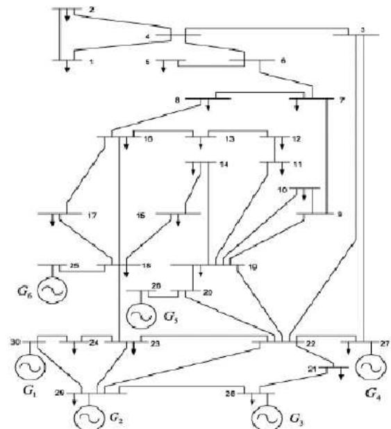
Fig. 13: Single line diagram of IEEE 30-bus 6-generator test system.
