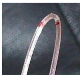
Fig. 2.1: Photograph of the tapered U-bent fiber probe.
