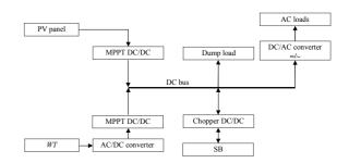
Fig. 1: Autonomous HGPS schematic diagram.
