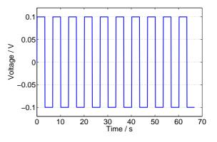
Fig. 2: Voltage square wave that the memristor measured in Figure 1 was subjected to.
