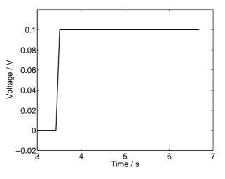
Fig. 5: An example of a voltage step as applied to a memristor.
