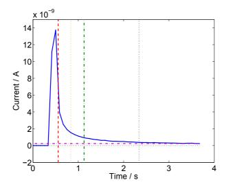
**Fig. 6:** An example Spike. Red dashed line:  $\tau_{50}$ ; orange dotted line  $\tau_{90}$ ; green dot-dashed  $\tau_{95}$ ; blue dotted  $\tau_{99}$ . Horizonal purple dot-dashed line is  $i_{\infty}$  and the spike height is  $i_{0}$ .
