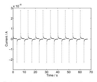
**Fig. 1:** Current spikes recorded from a memristor subjected to the voltage square wave in Figure 2. The spike heights are highly repeatable and qualitatively resemble neuronal spikes.
