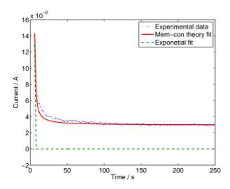
**Fig. 8:** A longer-term spike response fit by the mem-con theory. The mem-con theory fits the experimental data well, the best result fitting the data with an exponential is added as a comparison. Blue dots: experimental data, red line: mem-con fit, green line: exponential fit to the spike.
