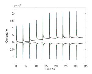
**Fig. 3:** The spikes for 5 successive runs up and then down the voltage staircase shown in Figure 4. The runs are coloured and overlap. The spikes are highly reproducible on successive runs
