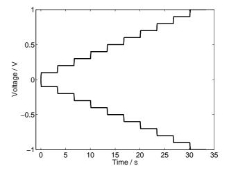
**Fig. 4:** Voltage ramps for Figure 3. 5 sets of positive voltage ramps-negative voltage ramps were run, to give the spike response in Figure 3.
