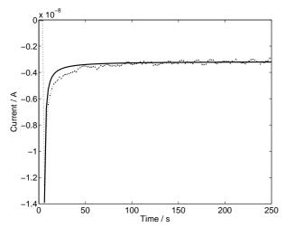
**Fig. 9:** A longer-term negative spike, demonstrating that the negative spikes are fit equally well by the mem-con theory. Blue dots: experimental data, red line: mem-con fit.
