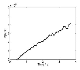
**Fig. 7:** The resistance profile for the memristor subjected to the voltage in Figure 5. Note that the 'zero' resistance is due to zero measured resistance as no voltage is applied, not a true zero resistance.
