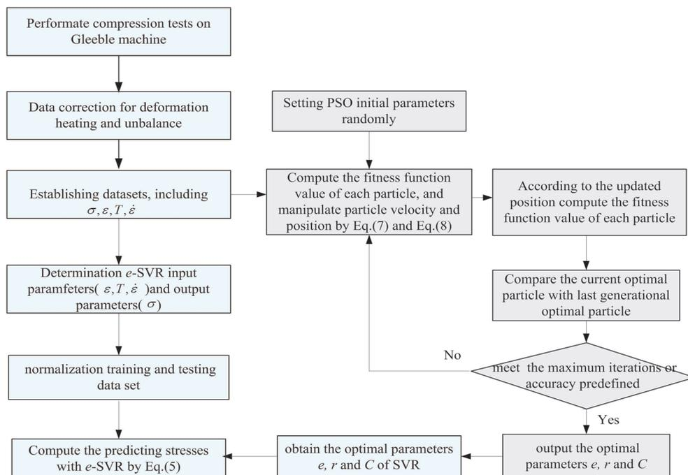
**Figure 2** Flow chat presenting model of high temperature flow stress of AZ80
