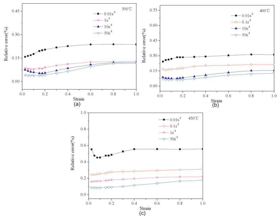
**Figure 5** Comparison of stress relative error of training samples obtained at (a)350°C,(b)400°C and (c)450°C
