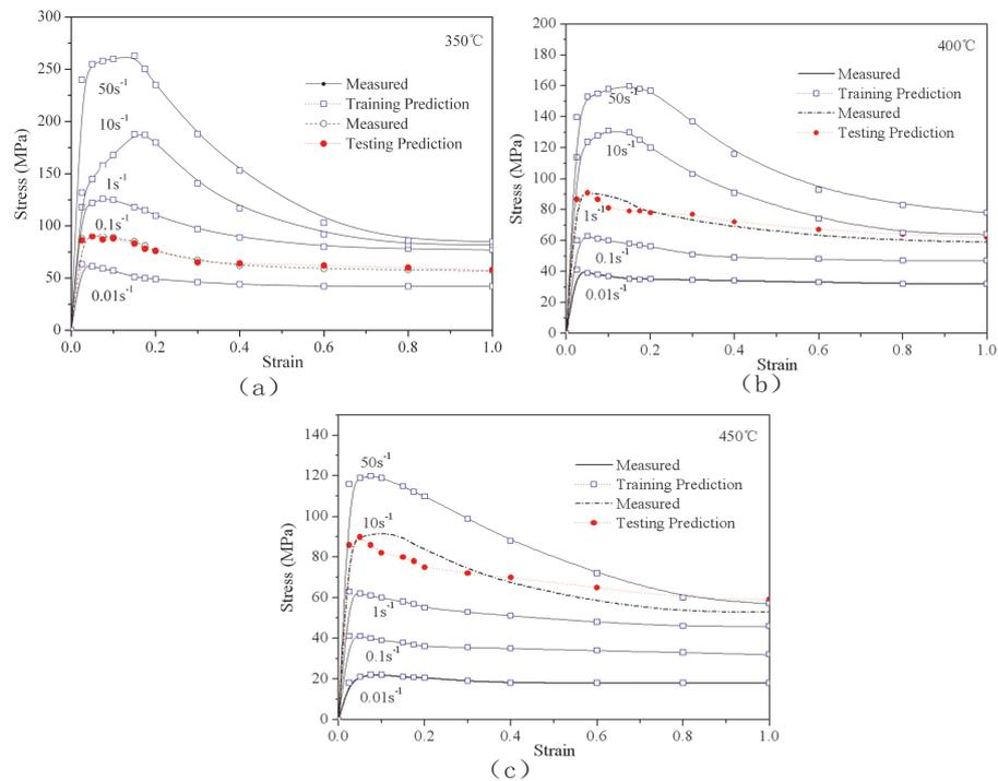
**Figure 4** Comparison of measured and predicted flow stresses between training and testing sets at (a)350°C,(b)400°C and (c)450°C
