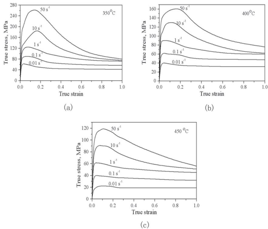
**Figure 1** True stress-true strain curve obtained at different strain rates and various temperatures, (a) at 350°C, (b) at 400°C, (c) at 450°C
