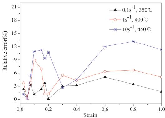
**Figure 6** Comparison of stress relative error of testing samples
