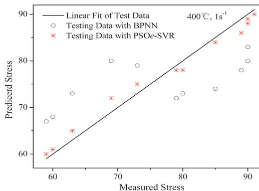
**Figure 8** Scatter plot for the testing samples of flow stress at 400°C,  $\dot{\epsilon} = 1s^{-1}$
