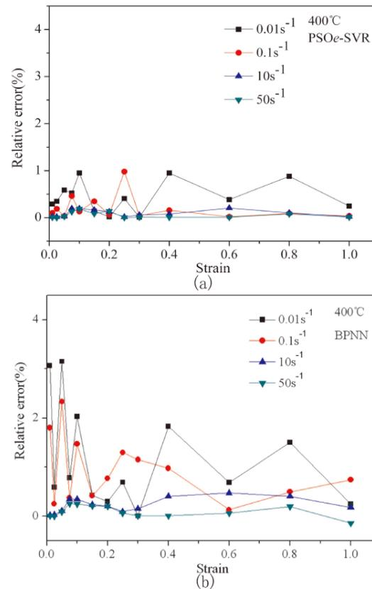
**Figure 7** Comparison of stress relative error of training samples obtained at  $400^{\circ}C$ ,  $\dot{\epsilon} = 1s^{-1}$  between (a) PSOe-SVR and (b) BPNN
