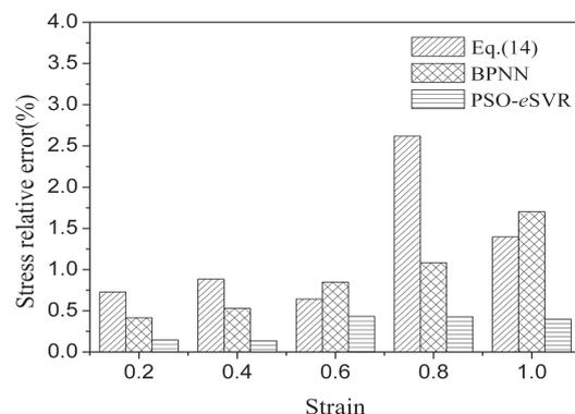
**Figure 9** Comparison of stress relative error obtained at 450°C and  $\dot{\epsilon} = 1s^{-1}$  using BPNN, PSOe-SVR and the constitutive equations
