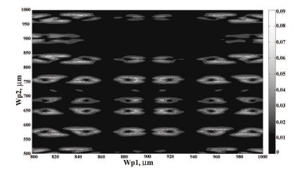
Figure 3.1: Dependence of ratio R on plates thicknesses
