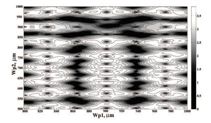
Figure 3.2: Dependence of average information losses L on plates thicknesses
