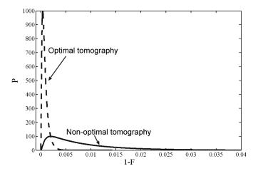
Figure 3.3: Dependence of density of distribution on the accuracy information losses 1 - F. Dot line corresponds to optimal set of plates (optimal tomography), solid line corresponds to non-optimal set (non-optimal tomography).
