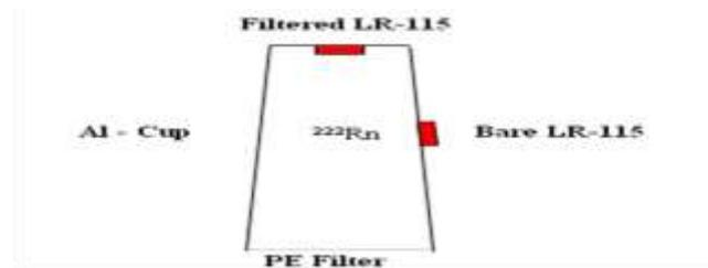
**Fig. 4:** Schematic diagram of the passive radon device [17].
