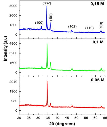
**Fig 1:** XRD patterns of the deposited ZnO thin films for different molarities.
