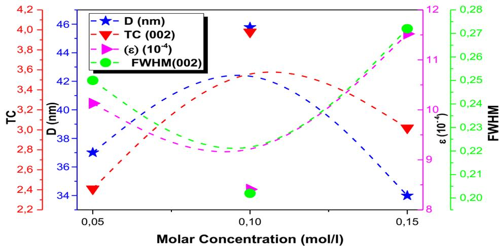
**Fig 4:** the average crystallite size (D), texture coefficient (TC), micro-strain ( $\epsilon$ ) and FWHM Of ZnO thin films prepared for different molarities.
