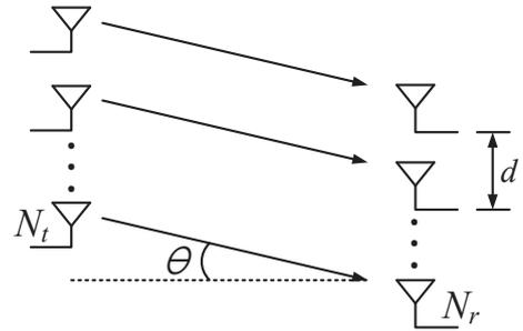
Figure 2 Wavefront impinging across MIMO array
