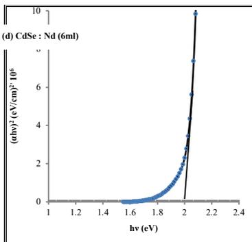
**Fig.4(d):** Tauc's plot for CdSe : Nd, 6ml.
