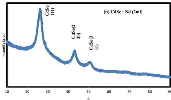
Fig.1 (b): XRD pattern of CdSe :Nd, 2ml.
