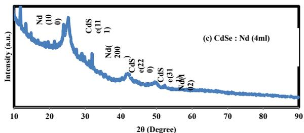
Fig.1 (c): XRD pattern of CdSe :Nd, 4ml.
