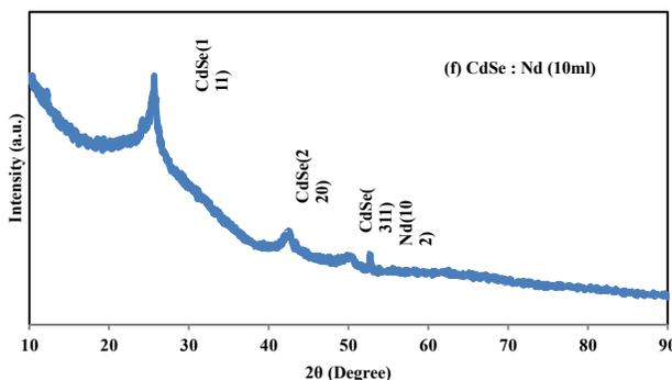
**Fig.1 (f):** XRD pattern of CdSe :Nd, 10ml.
