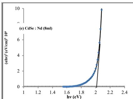
**Fig.4(e)** Tauc's plot for CdSe : Nd, 8ml.
