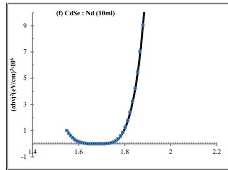
**Fig.4(f):** Tauc's plot for CdSe : Nd, 10ml.
