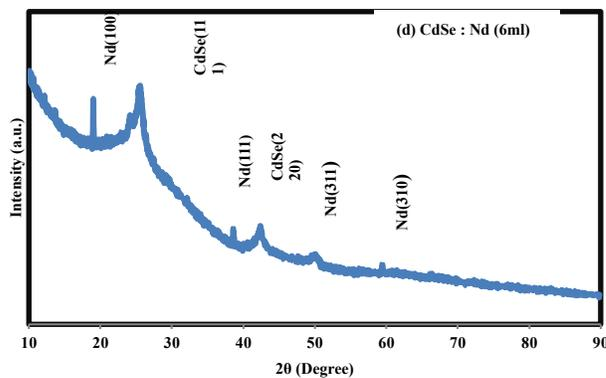
**Fig.1 (d):** XRD pattern of CdSe :Nd, 6ml.
