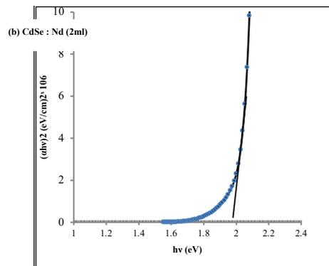
Fig.4(b): Tauc's plot for CdSe : Nd, 2ml.
