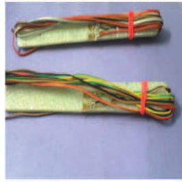
Fig. 3: Test Specimen with strain Gauge
