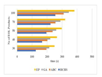
**Fig. 4:** Comparison of disassembly time at variable no. of E-O-L products
