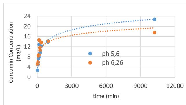
**Figure 6.** Release kinetics of curcumin from okra gum coated zein films at different pH values.
