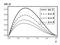
**Fig. 2:** Effect of viscoelastic second grade parameter  $\alpha$  on secondary velocity profile w(t,y).
