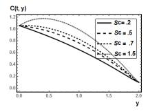
**Fig. 19:** Effect of Schmidt parameter Sc on concentration profile C(t,y).
