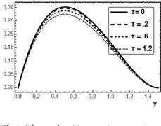
**Fig. 6:** Effect of thermophoretic parameter  $\tau$  on primary velocity profile u(t,y).
