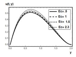
**Fig. 13:** Effect of Eckert parameter Ec on primary velocity profile u(t,y).
