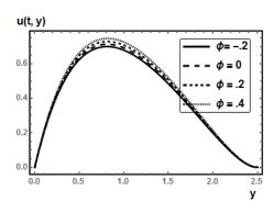
**Fig. 5:** Effect of heat source parameter  $\phi$  on primary velocity profile u(t,y).
