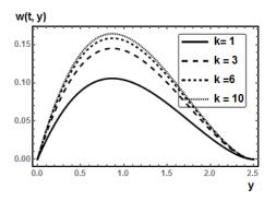
**Fig. 10:** Effect of Darcy parameter K on secondary velocity profile w(t,y).
