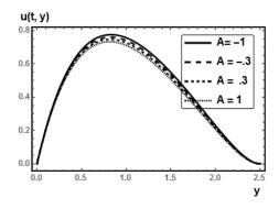
**Fig. 7:** Effect of suction parameter A on primary velocity profile u(t,y).
