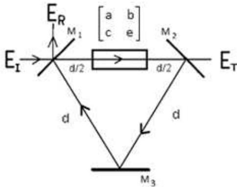
**Fig. 1:** Ring phase conjugated laser resonator with chaos generating element.
