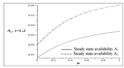
**Fig. 7:** Steady state availability  $A_i$  versus repair rate  $\mu$ , i=1,2
