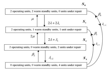
Fig 2: State transition diagram of 2-out-of-4:G warm standby parallel repairable system
