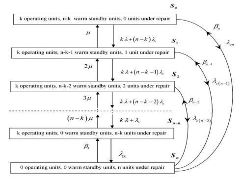
Fig. 1: State transition diagram of the k-out-of-n:G warm standby parallel repairable system
