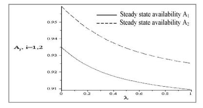
**Fig. 6:** Steady state availability  $A_i$  versus failure rate  $\lambda$ , i=1,2
