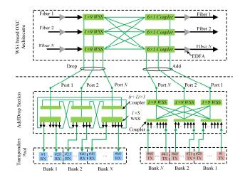
**Fig. 1:** CDC ROADM with OXC and add/drop sections where the nodal degree N equals 3, the connecting branches r is N-1, here equals 2, S equals 23, 40 wavelengths per fiber and 50% add/drop ratio, RX: Receiver (in blue), TX: Transmitter (in red).
