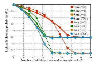
**Fig. 3:** The light-path blocking performance of the Italy network. (Ana: Analysis (dashed curve), Sim: Simulation (solid curve), 1.5 Erlang per node pair, r denotes the number of connecting branches, CDC case: where r equals N-1, where the max ( $N_i$ ) is 9).
