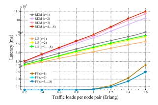
**Fig. 4:** Latency in function of the traffic loads per node pair. Simulations show comparisons among three bank selection algorithms: Random (RDM), Least Used (LU) and First Fit (FF) with different connecting branches r, from 1 to N-1 respectively. N is denoted as 9 for Italy network topology.
