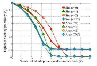
**Fig. 2:** The light-path blocking performance of the NSFNET network. (Ana: Analysis (dashed curve), Sim: Simulation (solid curve), 1.5 Erlang per node pair, r denotes the number of connecting branches, CDC case: where r equals N-1, where the max ( $N_i$ ) is 4).
