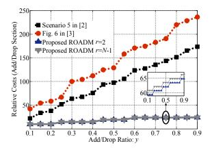
**Fig. 5:** Relative costs comparisons among three ROADMs: Scenario 5 in [2], Fig.6 in [3] and the proposed ROADMs against various add/drop ratios with two different connecting branches r scenarios, equals 2 and N-1 respectively. N is denoted as 4 here.
